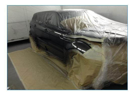
The 20-07 HS compliant Clearcoat was then mixed 2:1 with no thinner and applied through a 1.3 tip, with a 5 to 7 min. flash off between coats. It was baked for 35 minutes and gave an exceptional crystal clear durable high gloss.
