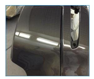
The clear plastic primer KFP.0014 was applied over a fully degreased bumper and the QUOSH water base coat was then applied . The bumper and the off side of the vehicle were then coated with the 2007 clearcoat with the applications as below.....
