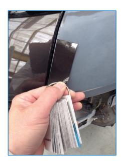
Once the vehicle colour has been established, the code is entered onto the IVAT software telling you the chip references and number of shades. With the colour selected, it is then mixed from the system. If accelerated drying is required, the Bi-Power accelerator, H2D.TTT1 is added to the mix.
