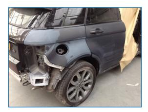
The Bumper is removed, and the and the offside panels are prepared and coated with the IVAT 2K Primer filler with etch - KFL.8888./7777 - Application is directly to bare metal, galvanised sheeting aluminium and hard plastics if required.
