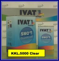
**KKL.5000 Anti scratch compliant acrylic clear coat supplied in 1lt. and 5lt.** It is mixed 2:1 with FK9.7777 hardener plus 10% RDL.777 thinners. Application through a 1.3 - 1.4 tip of 2 full coats with a 5 min flash off between coats, gives excellent flow out and a high gloss durable gun finish.
